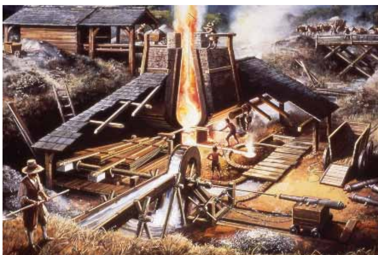
A blast furnace powered by waterwheel © Mike Codd - West Sussex County Council
